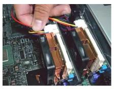
Connecting the power cable to the second PL-P3/SMP.
